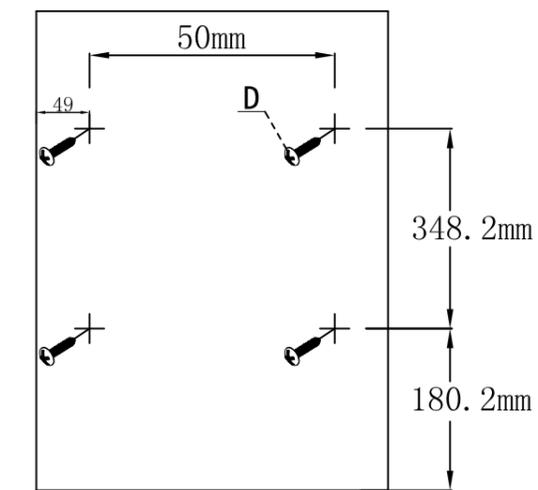
screw hole locating according to paper mould
